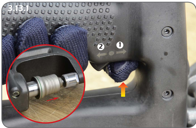
3.13.1 Press the rocker switch (pos. 1) on the hydraulic actuator towards the rivet clamp to extend the piston.
